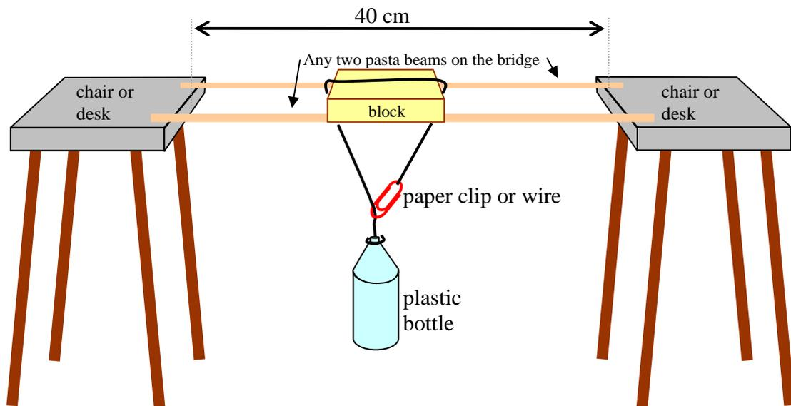
The reason for hanging the weight from the block (rather than attaching the string directly to the pasta) is to allow the weight to be spread across separated beams without causing beams to be pulled together horizontally.
