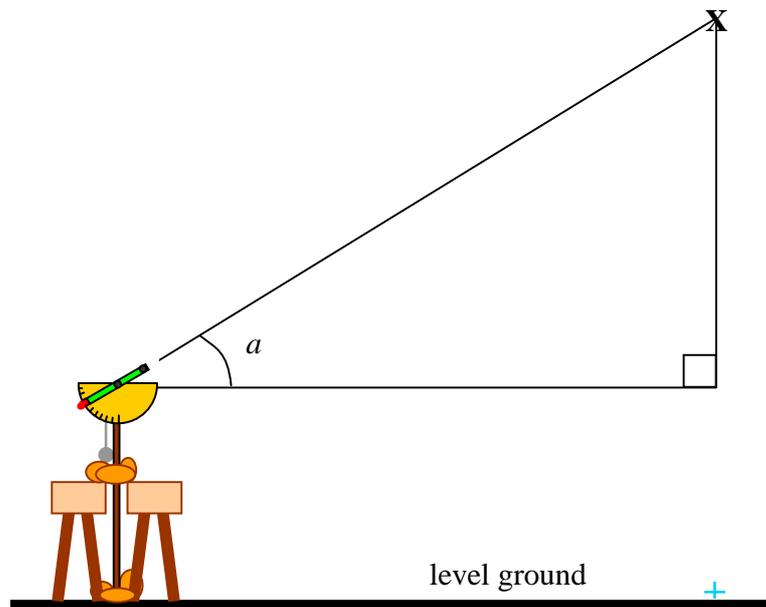
To measure  $a$ , the angle of the straw is adjusted until you can see the X
